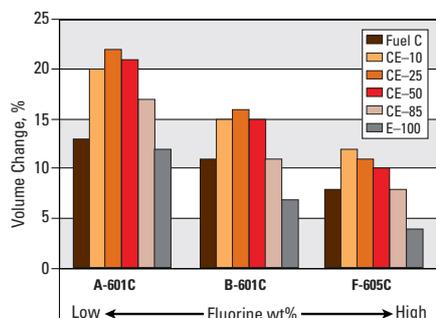
ASTM D 471-98—all fuel testing was conducted in sealed one liter 316 stainless steel Parr pressure vessels
