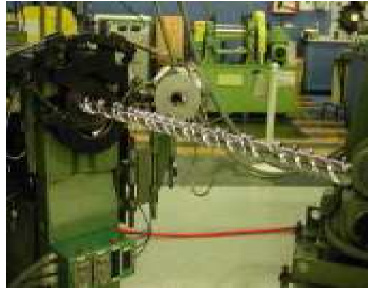
Barrier screw used for optimal FKM extrusion
